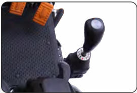
Single Joystick with Positive Locking System (Comfortable Positioning for Operation)
